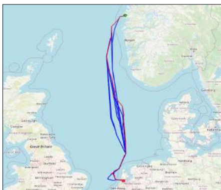
Figure 4: ETA optimised route in the North Sea, accounting for weather conditions during navigation.
